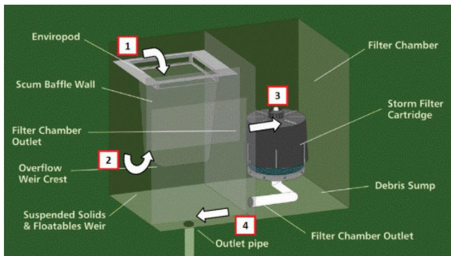
**Figure 2. Schematic of the SYSTEM treatment train.**
