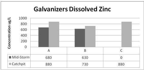
Fig 7. Galvanizing Facility Dissolved Zinc Concentrations
