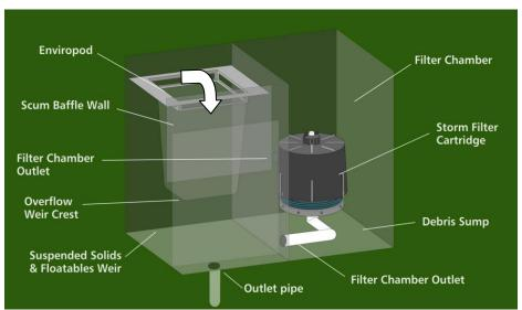
Fig 1. Kuranda SFEP: Treatment train layout.
