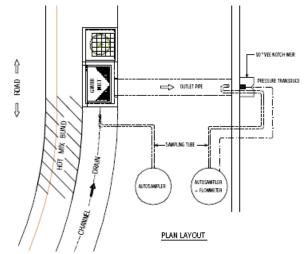
Fig 2. Kuranda SFEP: Experimental set-up
