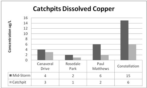
Fig 9. North Shore Catchpits Dissolved Copper Concentrations
