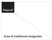
Based on a comparison of a traditional designed raingarden (k=0.3-0.75m/d) and the Filterra® (k=2.5m/h).
